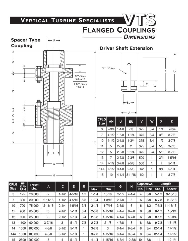
\*Note: Minimum dimensions required for coupling installation. - Check motor dimension.
